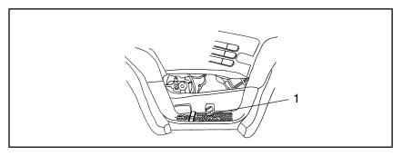
Your Polaris ATV has a foot brake (1) provided as a safety feature. It is located on the inside of the right floor board and is operated by the right foot. It is intended as a backup to the main brake system, especially if the main system becomes inoperative.
